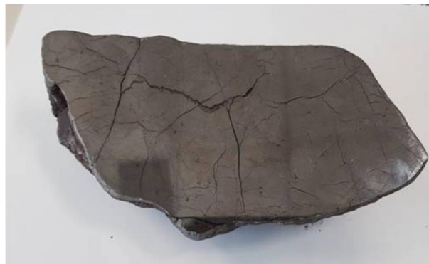
Hand specimen from Disko showing large interlocking nickel-copper PGE rich crystals of massive sulphide
